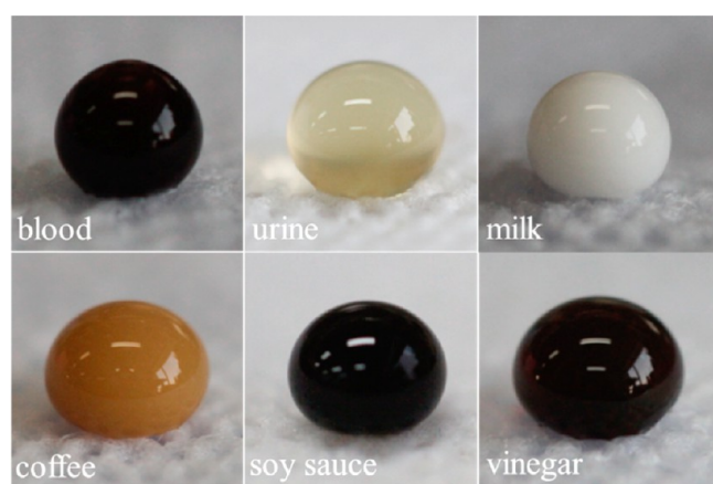
Figure 4. Digital photos of various liquid droplets of about 80 \mu\text{L} in volume resting on PP nonwoven fabrics treated by solvent B for 10 s at 80 °C.
